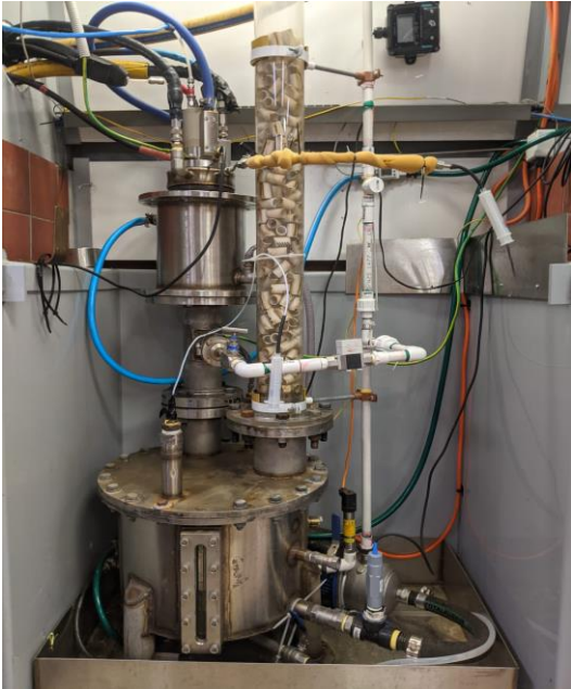
Plasma destruction: pilot plant, nominally 50 L/day feed
