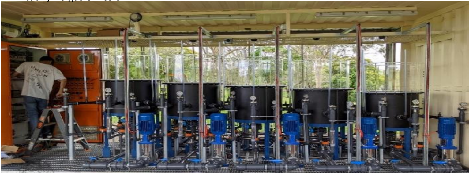
Foam fractionation concentration: demonstration plant, nominally 20-t/day feed water
