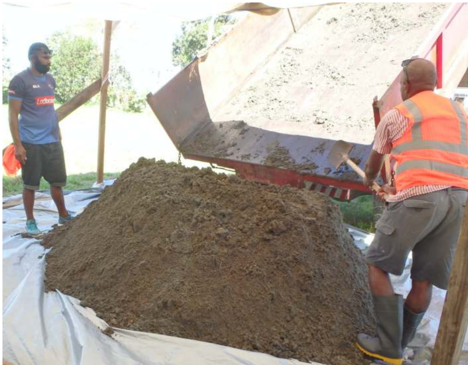
Plate 6 – Sample being prepared for drying and bagging
