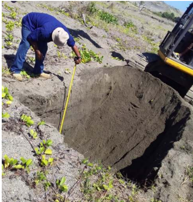
Plate 2 – Depth measurement prior to sample collection
